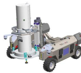
Figure: preliminary design of the mobile quantum gradiometer within FIQUgS project (left) and laboratory atomic gravi-gradiometer of SYRTE (right)
