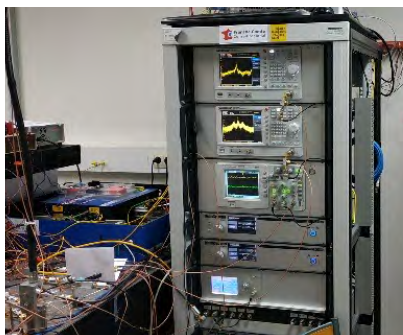
Optical to \mu wave (H-Maser, CSO) comparison \approx 10^{-15} Stability transfer from 1.55 \mu m to 871 nm ( Yb^+ clock laser)
